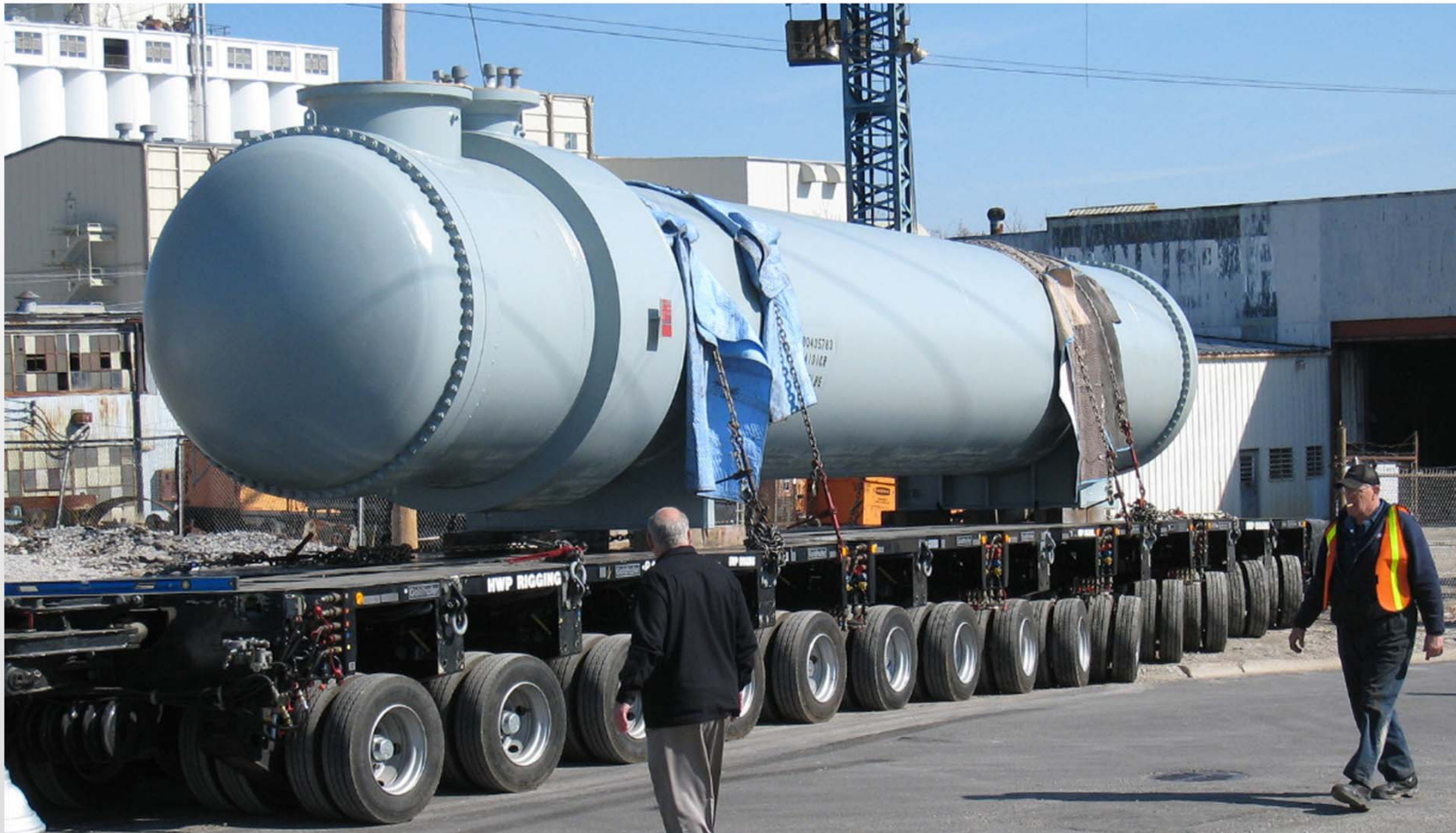
79-492 NEN Propylene Refrigerant Desuperheating/Condenser (172,000 lb)
