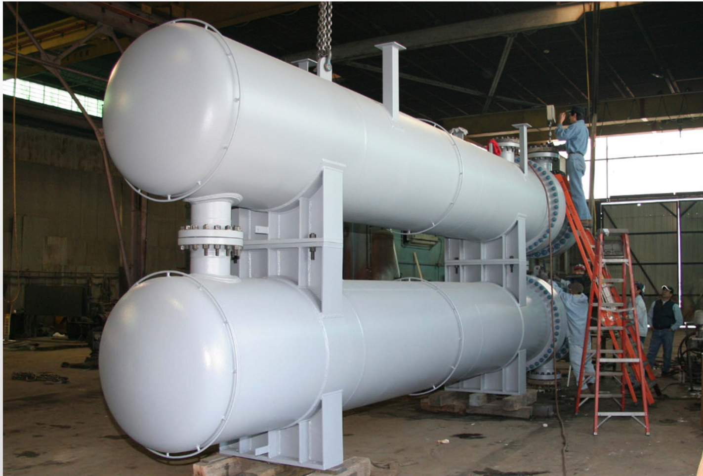
Triple Stack 43-240 CEU Crude Cross Exchangers (155,000 lb Total)
