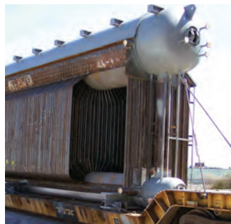
250,000 lb/hr 725 psig superheated boiler system.
